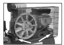
Figure 11. Belt Guard and mounting bolts.
